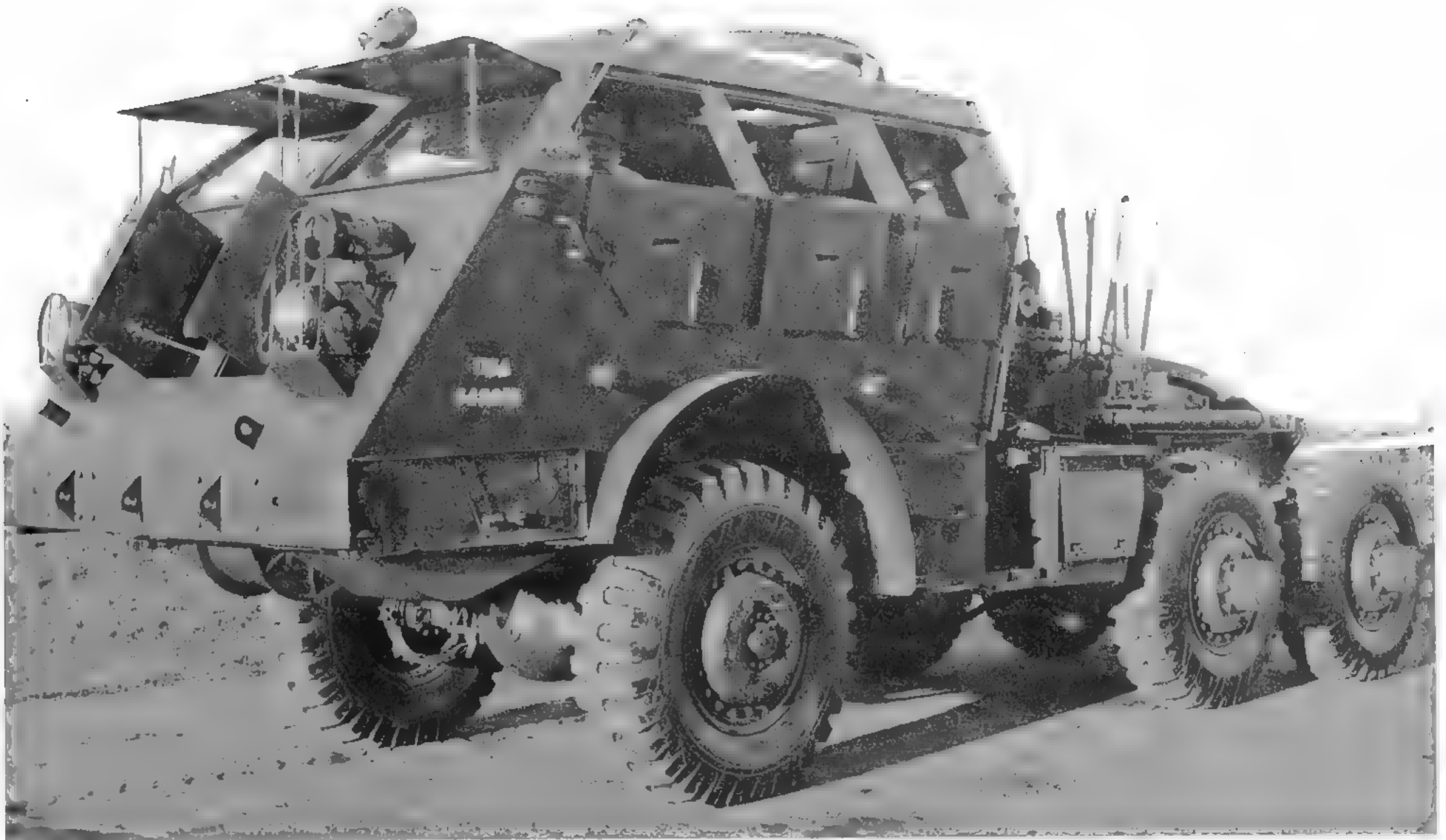
The shiny M26 shown in this 1949 photograph has had its outer dual wheels removed. Barely visible behind the front bumper is the drum for the 35,000-lb.-capacity front winch. (U.S. Army photo)
